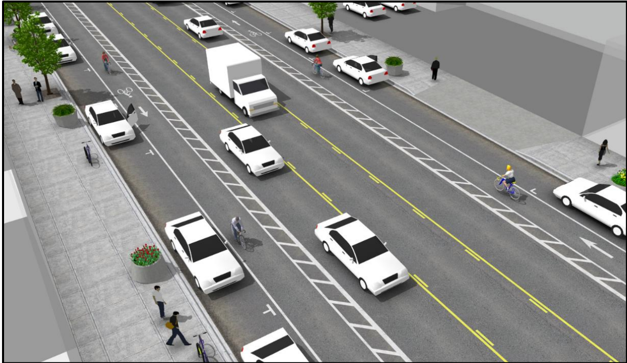
Figure 3-5: Example of Buffered Bike Lanes
